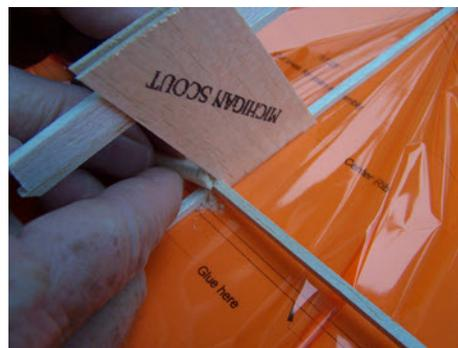
5.4 Put a drop or two of the Thin CA glue to complete the forming of the fillet. The glue will auto cure. The fillet is there to make a strong joint where 2 pieces of wood have just a line contact (where they touch forms a line).
